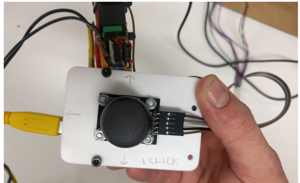
fig.15 The joystick, assembled with all electronic parts
